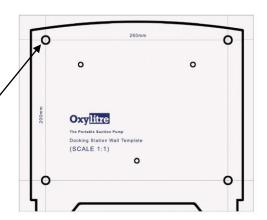
e. Remove the paper template, and depending on the type of fixtures selected, prepare the mounting holes at each point marked.
